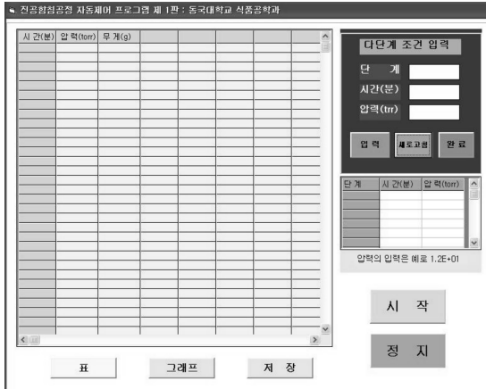
Fig. 2. Typical computer program window used for vacuum impregnation equipment.
