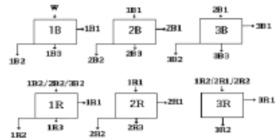
Fig. 2. Schematic diagram of mass streams in milling process in Buhler automatic laboratory mill. 1B3, 1B-flour; 2B3, 2B-flour; 3B3, 3B-flour; 1R3, 1R-flour; 2R3, 2R-flour; 3R2, 3R-flour; 3B1, bran; 3R1, shorts; the others, intermediate masses.
