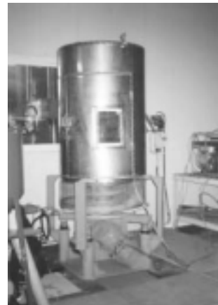
Fig. 10. Photograph of spiral vibration dryer
