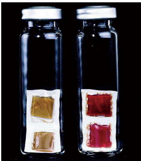
Fig. 5. Myoglobin-based films that change their colors from brown to red at  $\geq 0.13$  mg/L of hydrogen sulfide concentration. Reproduced with permission from Elsevier, License no: 5801981452986.
