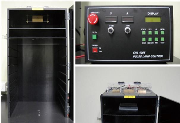
Fig. 1. Schematic diagram and photography of the intense pulsed light treatment system.
