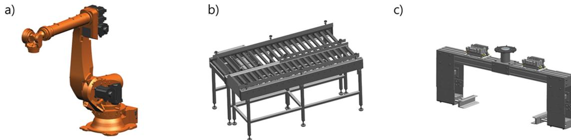
Fig. 2. 3D modeling used in robot-based 3D simulation. (a) Articulated robot, (b) Conveyor machine, (c) Gripper.
