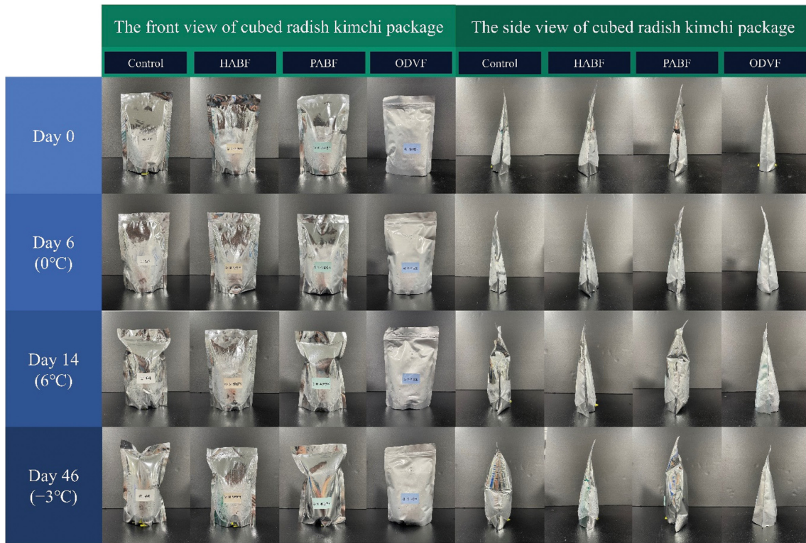
Fig. 6. Appearance of different packaging films for cubed radish kimchi during storage under altering temperature conditions.
