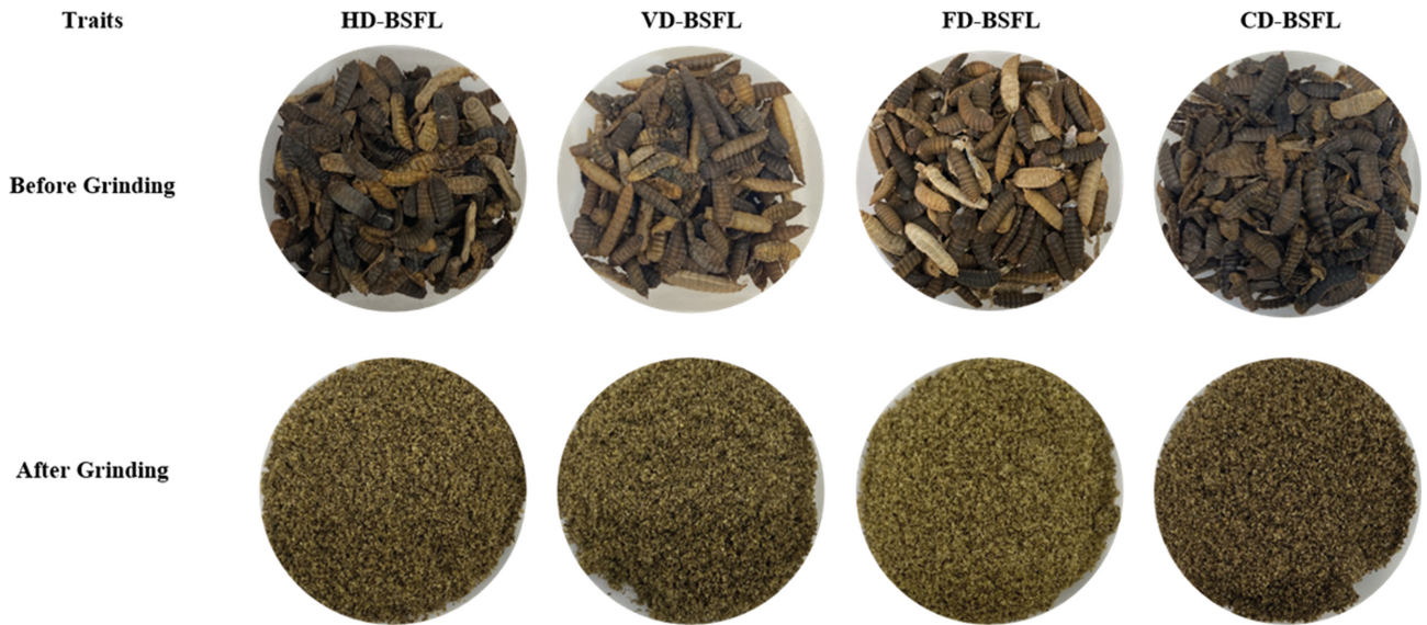
Fig. 2. Appearance of dried black soldier fly larvae dried by different method. (HD-BSFL) Hot-air drying black soldier fly larvae, (VD-BSFL) Vacuum drying black soldier fly larvae, (FD-BSFL) Freeze drying black soldier fly larvae, (CD-BSFL) Combined drying black soldier fly larvae.
