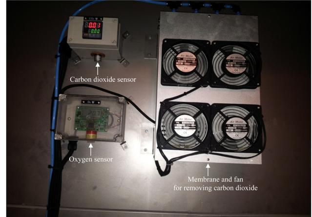
Fig. 3. Oxygen and carbon dioxide sensors in the CA container.
