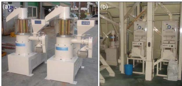
Fig. 5. Photographs of vertical rice mill system with an abrasive & friction roller: (a) final vertical rice mill developed in this study, (b) a vertical rice mill system installed (arrow) in the rice process complex.
